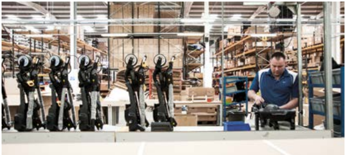
■ Every Powakaddy trolley is assembled by hand at its factory in Sittingbourne, Kent. Each model is built using the same basic chassis.
