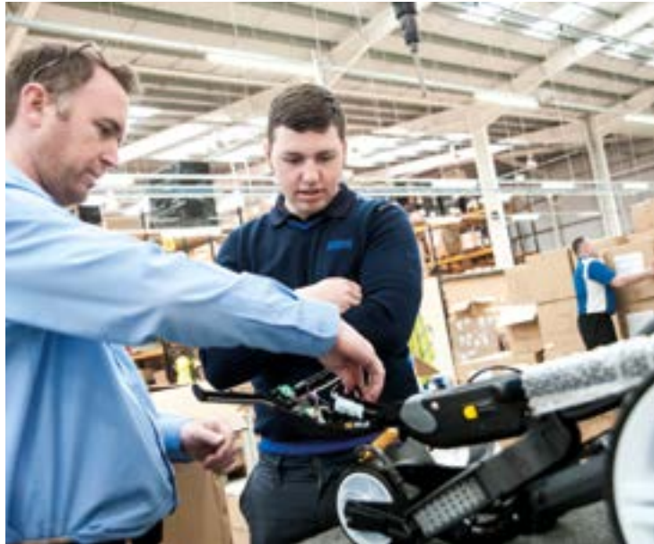
■ Every Powakaddy trolley is assembled by hand at its factory in Sittingbourne, Kent. Each model is built using the same basic chassis.
