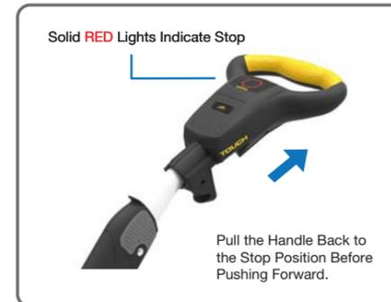
During normal use on course the isolation switch is not required, unless leaving the trolley unattended for long periods, the handle will hold in the stop position. Note: the stop position is not a parking brake, the trolley drive system will still freewheel on slopes and hills. For safety always come to a stop on flat ground or park across the slope to prevent accidental operation or the trolley rolling unpowered.
